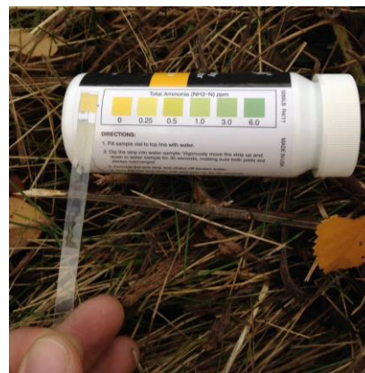
Figure 5 - Matching up the colour of the test strip with the colour coding on the bottle
